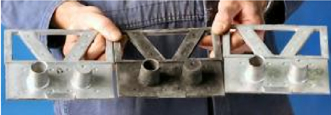
A display of three test castings, which, from left to right, are: 1. As cast (left), 2. Conventional heat treatment (middle), 3. Heat treated using the new procedure (right). (Credit: Mark Fergus, CSIRO)
